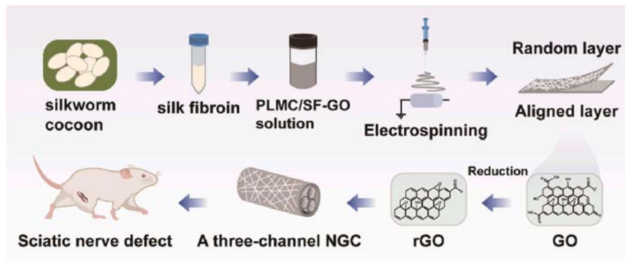
Fig. 2. Schematic illustration of the three-channel PLMC/SF-rGO NGCs and its application in repairing sciatic nerve defects in rats.
