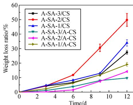
Fig. 8 The degradation of hydrogels.
