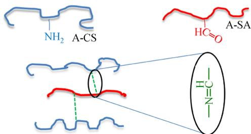
Fig. 4 The Schiff's base reaction between aldehyde group of A-SA crosslinking amino group of A-CS.
