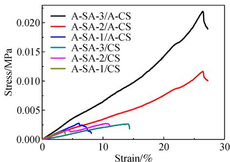
Fig. 7 The lap shear strength of porcine skin adhered by hydrogels.
