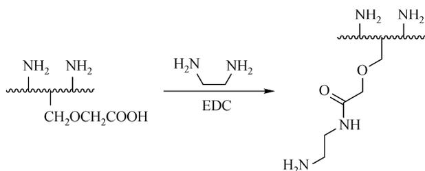
Fig. 3 The modification scheme of A-CS.
