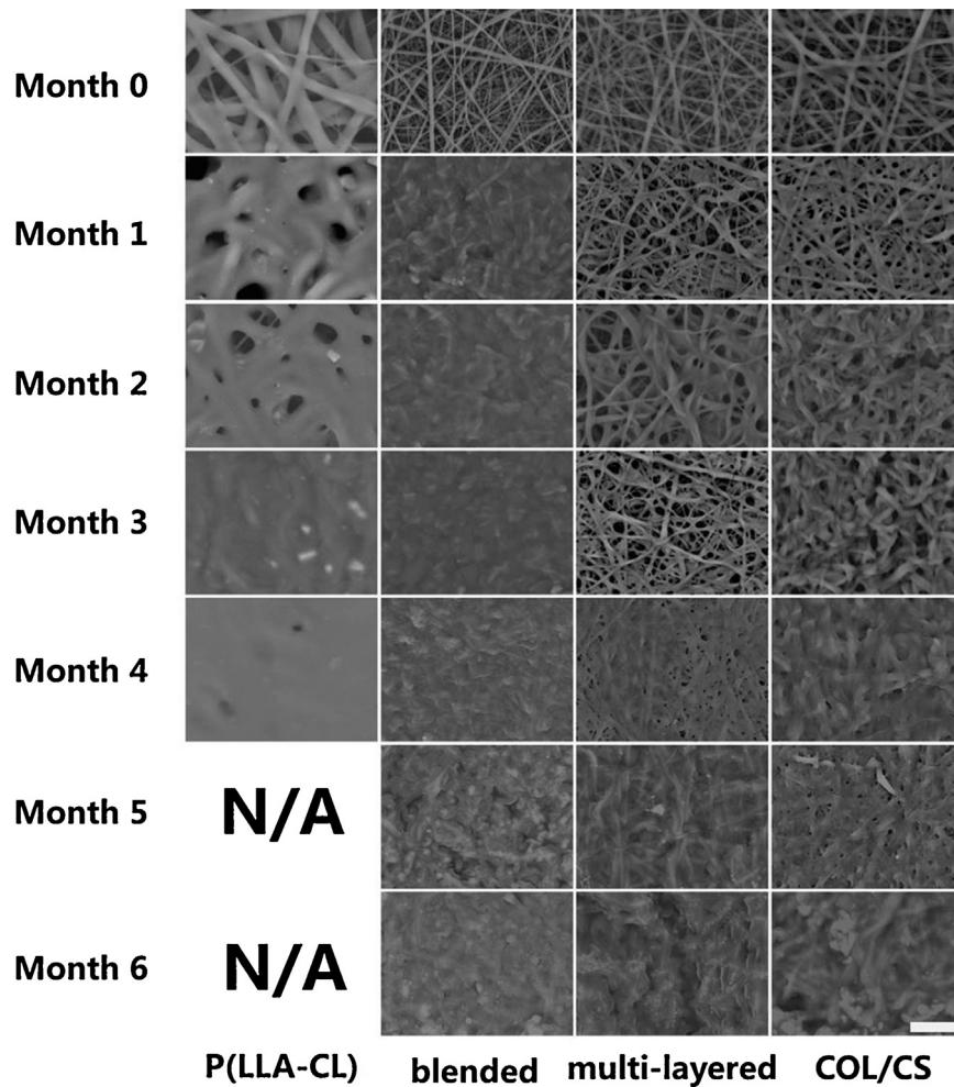
**Fig. 6.** Scanning electron micrographs of different scaffolds after biodegradation for different periods; bar = 10  $\mu\text{m}$ .
