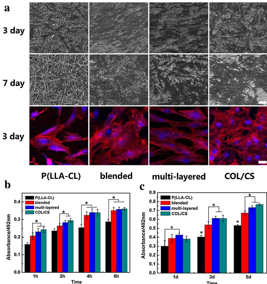
**Fig. 5.** (a) Scanning electron micrographs of hSMCs on different scaffolds after culturing for 3 and 7 days, and confocal images of hSMCs on different scaffolds after culturing for 3 days; adhesion and proliferation of hSMCs after culturing in 8 h (b) and 5 days (c); bar = 25  $\mu$ m.
