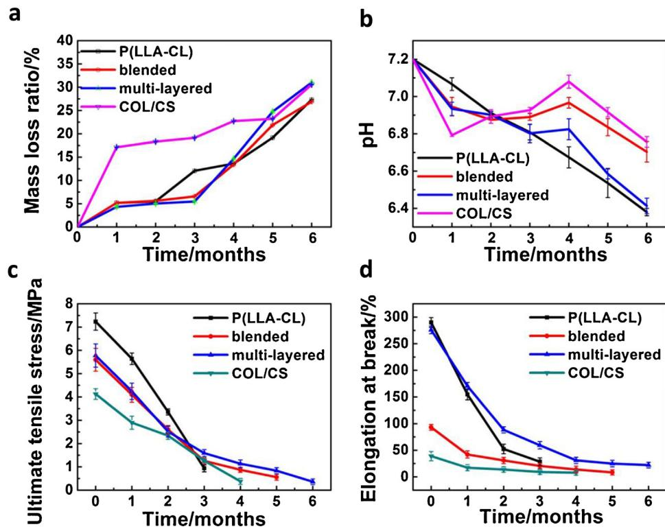
**Fig. 7.** Mass loss percentage (a), pH value change (b), ultimate tensile stress (c), elongation at break (d) of different scaffolds after biodegradation for different periods.
