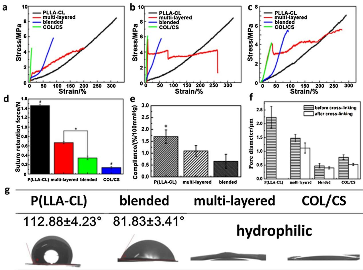
**Fig. 3.** Stress-strain curves of different electrospun scaffolds before cross-linking (a), after cross-linking in dry state (b) and in wet state (c); (d) suture retention force of the scaffolds with similar thickness; (e) compliance results of electrospun scaffolds in wet state; (f) pore diameter before and after cross-linking; (g) water contact angle of electrospun scaffolds.
