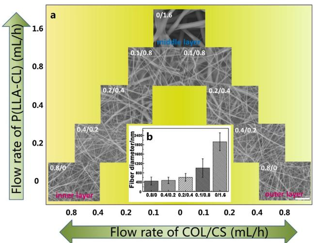
**Fig. 2.** (a) SEM images of different layers; (b) fiber diameter distribution of different layers; bar = 10 μm.
