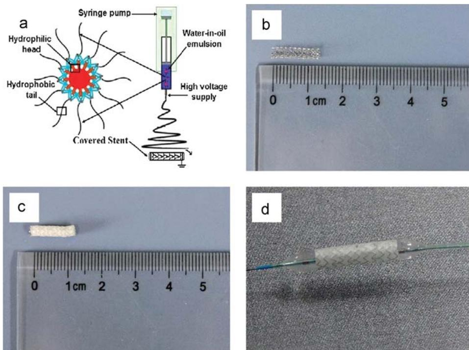
Fig. 1. The scheme of the fabrication of heparin loaded covered stent (a) and digital images of bare metal stent (b), covered stent (c) and expanded covered stent (d).
