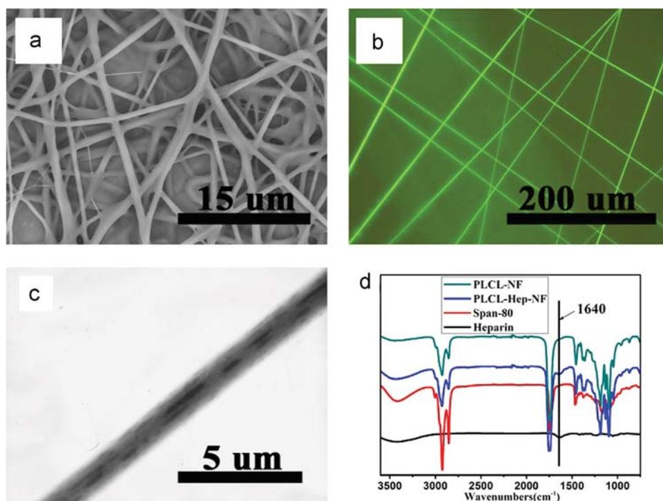
Fig. 2. SEM image (a), FM image (b), TEM image (c) of PLCL-Hep-NF and FTIR spectra of PLCL-NF, PLCL-Hep-NF, Span-80 and Heparin (d).
