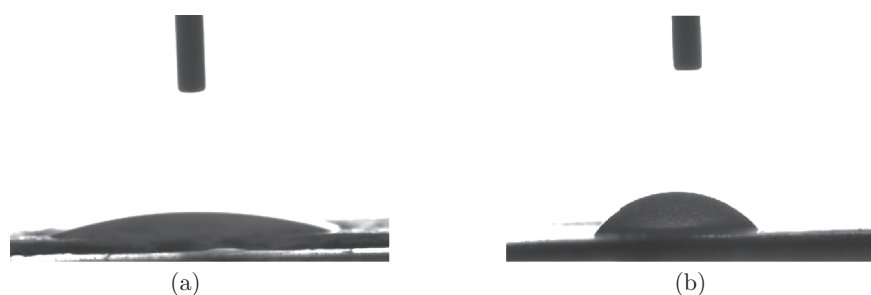
Fig. 3: Images of the static contact angles of nanofibrous membranes measured by a contact angle goniometer ( n = 6 ). (a) Collagen; (b) Collagen-chitosan
