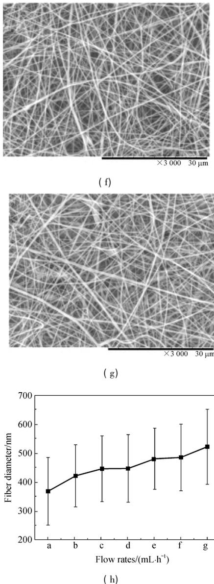
Fig. 2 SEM images of COL/CS with different flow rates ( ( a ) 0. 1 ; ( b ) 0. 3 ; ( c ) 0. 5 ; ( d ) 0. 7 ; ( e ) 1. 0 ; ( f ) 1. 5 ; ( g ) 2. 0 ) and average fiber diameter ( h )
