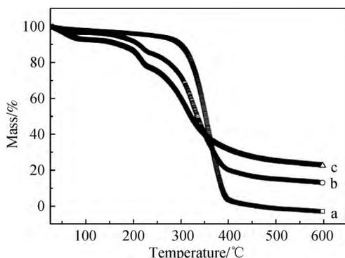
Fig. 5 TG curves of P( LLA-CL) ( a ) , composite ( b ) and COL/CS ( c ) scaffolds
