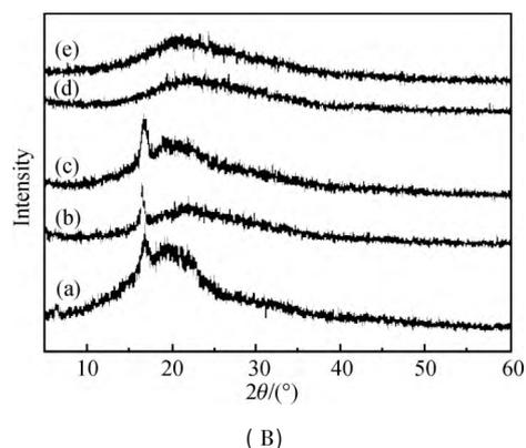
Fig. 4 FTIR-ATR spectra ( A ) and XRD curves ( B ) of P( LLA-CL ) ( a ) , composite ( b , c ) and COL/CS ( d , e ) scaffolds before GA crosslinking ( a , b , d ) and after GA crosslinking ( c , e )
