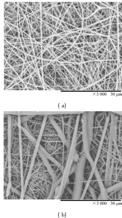
Fig. 3 SEM images of inner/outer layer ( a ) and middle layer ( b ) of multi-layered composite scaffolds
