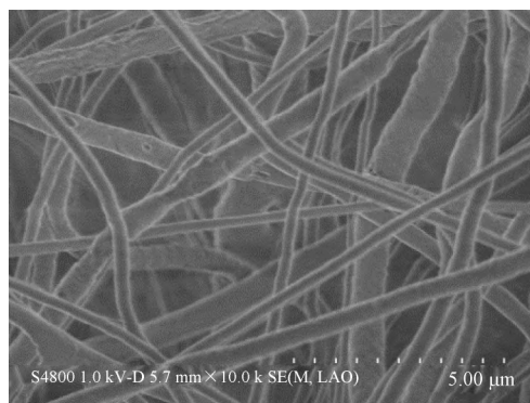
( l ) Film with 200 °C QDs ( scale bar 5 μm )
